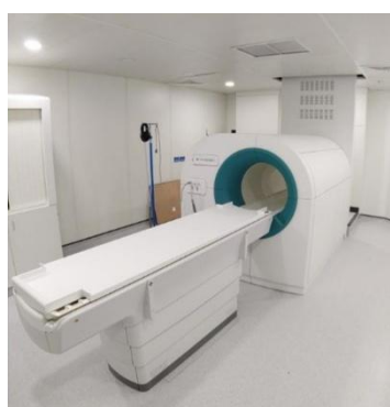
Left: New-generation FCI system assembled in the Aberdeen Royal Infirmary. Middle and right: typical magnitude images obtained for a 30-min field-cycling acquisition of the head from the previous FCI prototype (left: single-slice, 5 evolution times, 4 evolution fields, 80 \times 80 voxels) and the new FCI system (right: 8 slices, 5 evolution times, 9 evolution fields, 128 \times 128 voxels).
