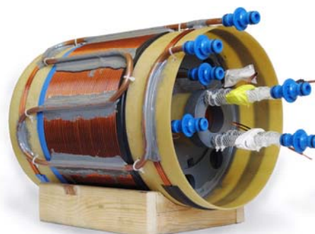
Fig. 2: Image of the 90mT FFC coil with cooling pipes. The outermost windings are the active shielding coil, the actual field coil is not visible.
